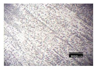
Fig. 5.5. Microstructure of weldment (100X)
