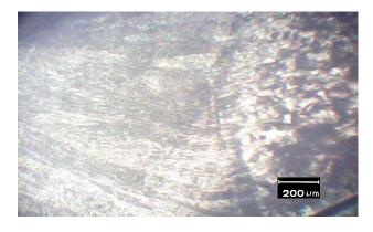
Fig. 5.4 Weld interface to corten steel (100X)
