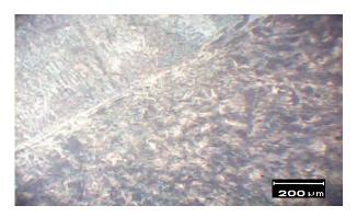
Fig.5.3 Weld interface to SS 304 (100X)
