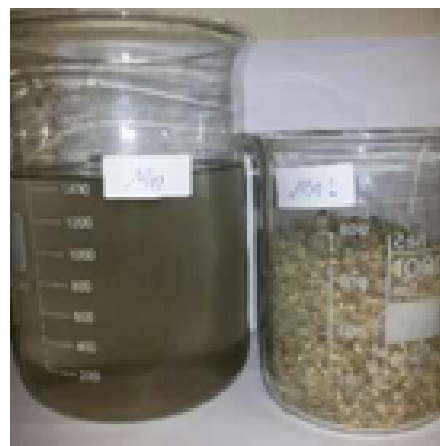
Fig. 4. The appearance LRW Sample after solidifying Process
