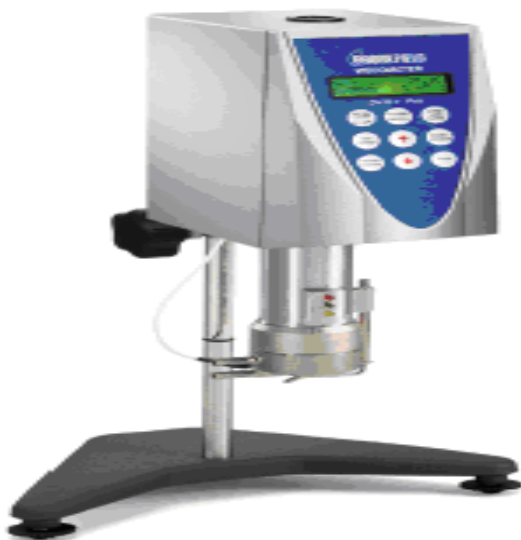
Fig. 3. Determination of viscosity by BROOK FIELD – SPINDLE NUMBER 2
