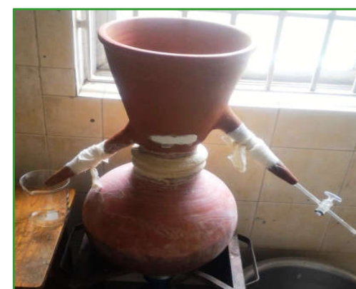
ppp Fig. D Distillation using Traditional Still
