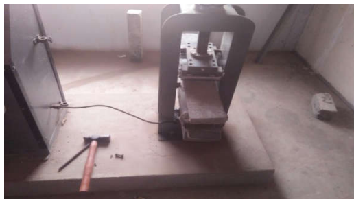
Fig. 2. Flexural test setup
