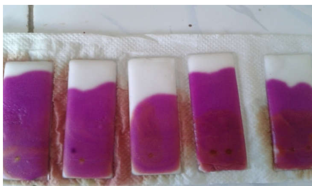
Figure 7 . Potassium permanganate treated TLC slides to confirm the presence of plant pigments
