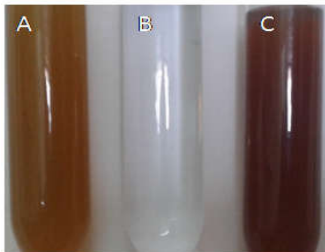
Fig. 3. Biosynthesis of nanoparticles (A) C. dentata leaf extract (B) AgNO_3 (C) AgNO_3 treated with C. dentata leaf extract.
