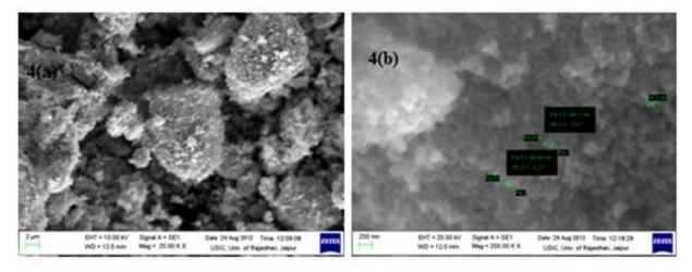
Fig. 4(a) and 4 (b) SEM images of THF mediated ZnO nanoparticles
