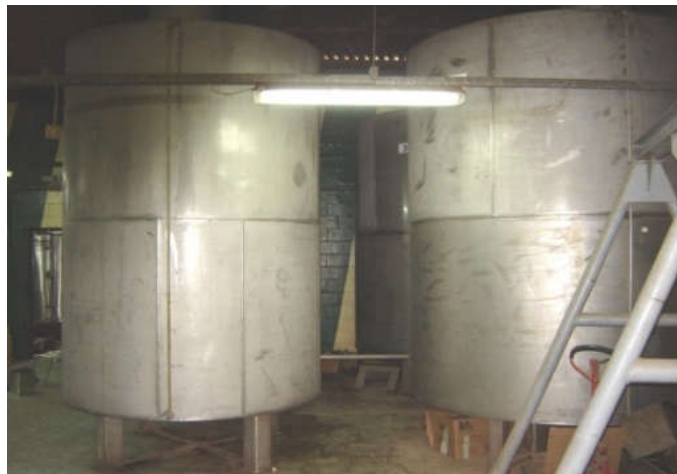
Figure 11. Olive oil is temporary stored into silo tanks
