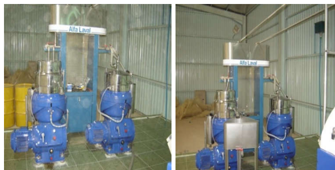
Figure 9. Olive oil separation from water (A), and water from oil (B)
