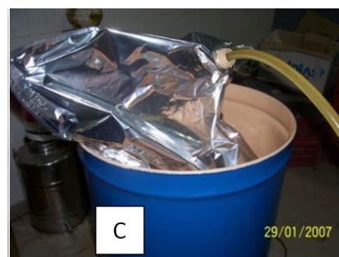
Figure 14. (A) Arrangement of Conical drums in the store, (B) Aseptic Bags, (C) Filling olive oil into aseptic bags
