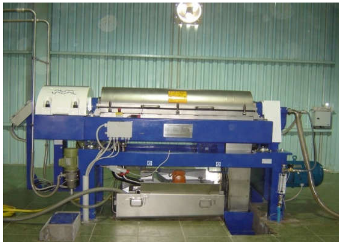
Figure 8. Decanter (Centrifuge) to separate olive paste from oil and water
