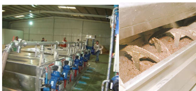
Figure 7. Olive paste mixing (malaxation) machines
