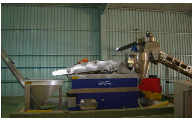
Figure 4. Leaves and light Impurities separator blower and Washing sink
